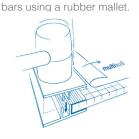
It is recommended that the top glazing bar is secured to the rafter with screws (gauge not exceeding 12g) at no greater than 1200mm apart. Once the next sheet is installed the second and subsequent top glazing bars can be fitted.
